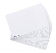
The iClass 2k/2 card from HID is a 13.56 MHz contactless smartcard designed for use with HID's door access control systems plus other compatible applications. The card contains 256 bytes (2k bits) of memory and is configured with 2 application areas. The first area stores the HID card number and the other is customisable for user requirements.
